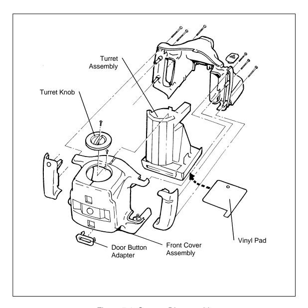
Figure 5-1 Camera Disassembly
